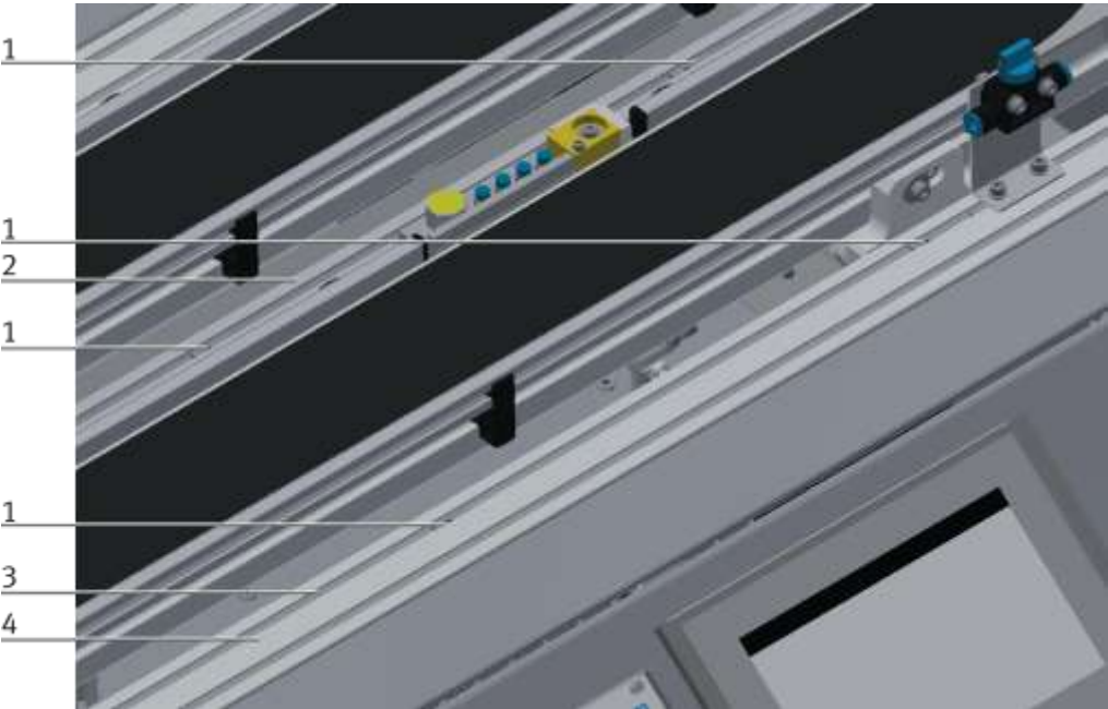
Positioning slot nuts / illustration similar
