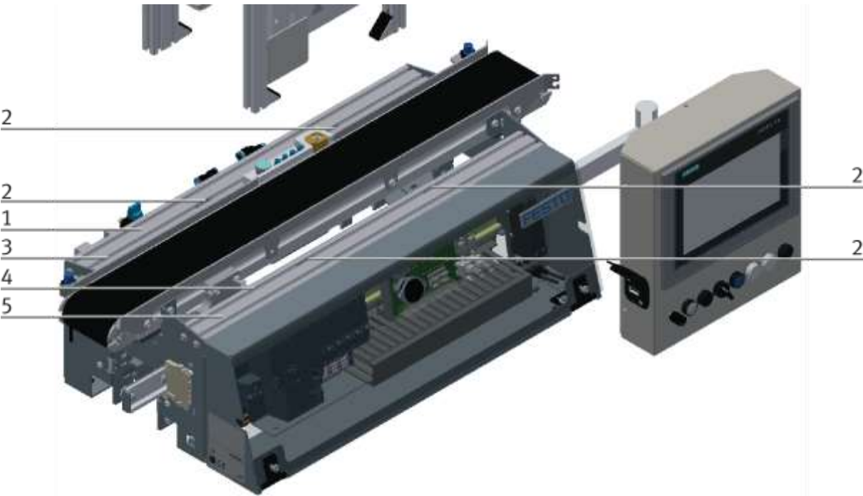
Positioning slot nuts / illustration similar
